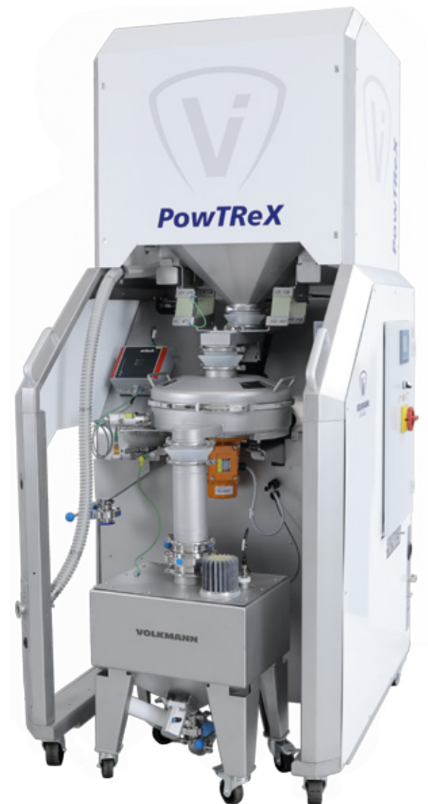
Fig.: The powder buffer has an effective capacity of 25 liters of metal powder.
