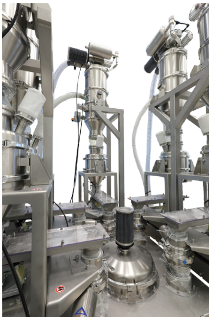
System at a food producer: Conveying and dosing five components of a recipe into a mixer.
